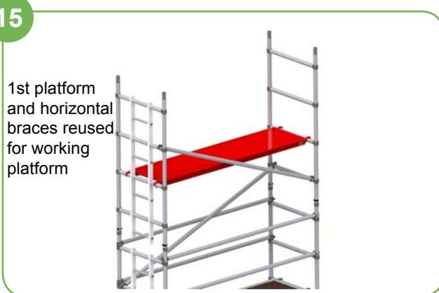
1st platform and horizontal braces reused for working platform
